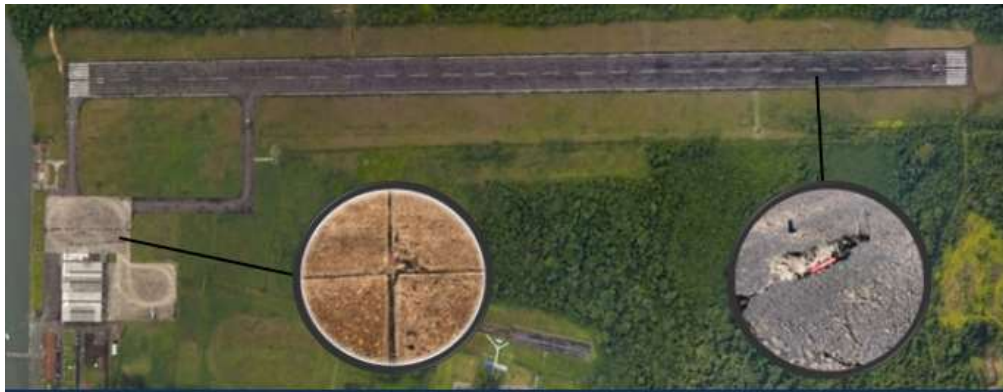
Figure 3. Satellite image of one of the evaluated airfields showing some distresses found on pavement surfaces. Source: authors.
