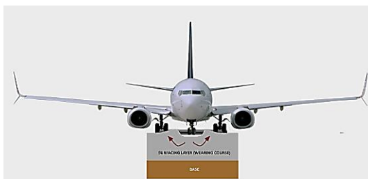
Figure 5 Rutting Shear deformation within the base layers of the pavement, near the surface. (Adapted from Dawson and Kolisoja, 2017).
